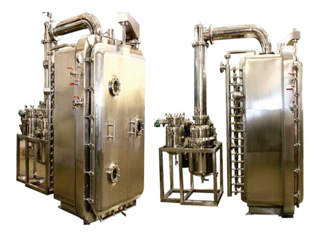
For temperature and oxygen sensitive products as well as in the processing of highly hygroscopic materials; drying under vacuum is required. Genesis (GPT) Vacuum Tray dryer is static tray dryer designed for exactly this purpose which works under vacuum conditions on conduction principle. This arrangement also supports in drying without contamination.
